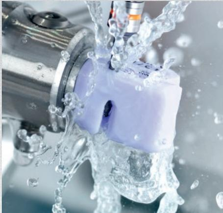
The patented Carving mode - allows glass and hybrid ceramics to be processed with a saving in time of approx. 60 %. This special grinding technique removes excess material in its entirety, thus bypassing the need to grind the block down to its actual geometry. The process, which to date is unique in dental CAD/CAM technology, results in massive time savings and is roughly equivalent to machining with two spindles (approx. 15 min/crown).
